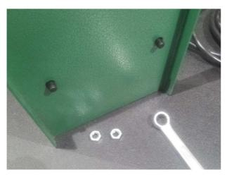
Remove the nuts holding the base on.
