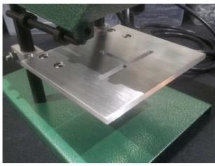
Raise the shelf up a couple of inches and tighten the ¼ nuts on the shelf supports. After the shelf supports are tightened you can tighten the shelf down to the shelf supports.
