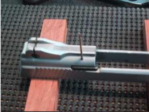
Remove the extractor by driving the pin out from the top.
