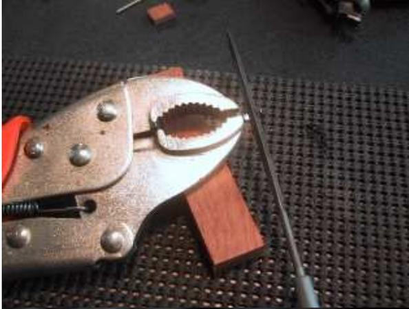
Use a triangle file to remove material. This will keep you from removing any on the face that grabs the rim. It's also better for getting in the corner. Do not remove material from the face. You need a Jewelers Loupe to do this right.
