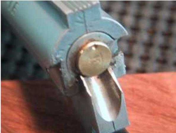
Insert a spent casing with strike mark up in normal fired position.
