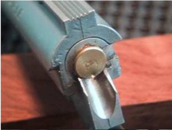
Try the spent casing with the strike mark in different positions. When the round is fired the area by the feed ramp will expand a little more so when you rotate it you can sometimes get a tighter fit for testing
